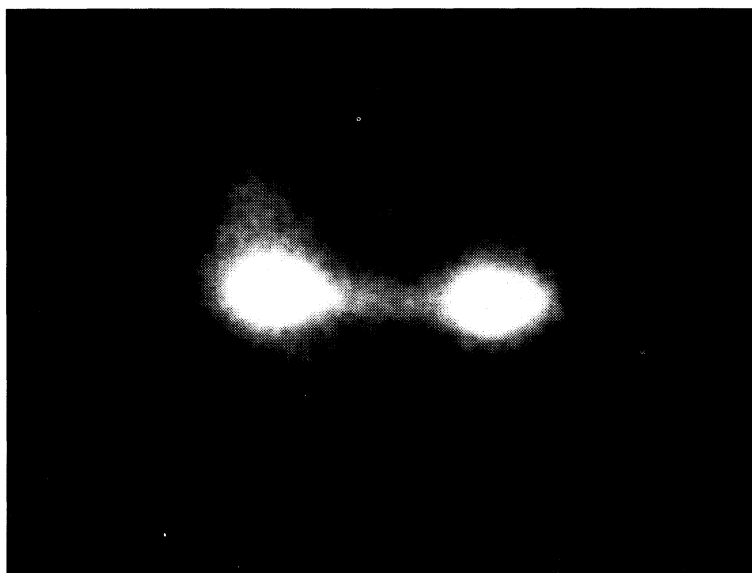
Figure 22. Electron diffraction pattern showing twin-related diffraction peaks in anorthoclase and diffuse streaks due to walls in between.
