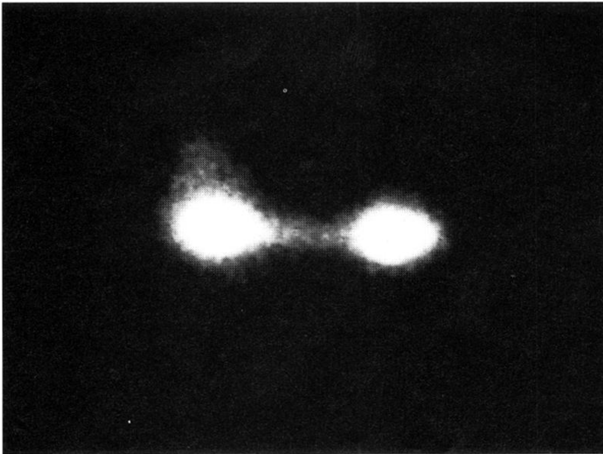
figure 22. Electron diffraction pattern showing twin-related diffraction peaks in anorthoclase and diffuse streaks due to walls in between.
